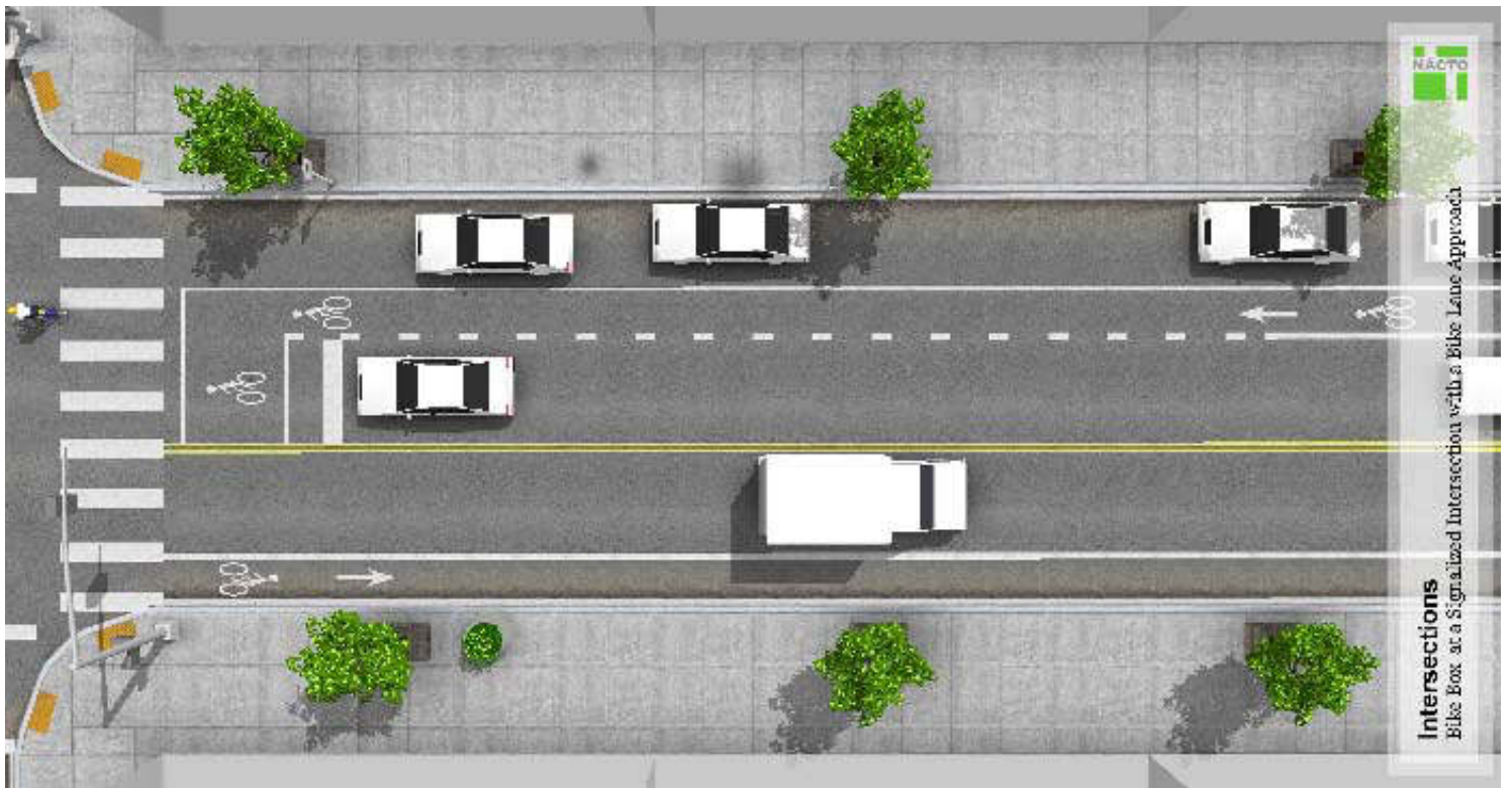
Intersections Bike Box at a Signalized Intersection with a Bike Lane Approach
