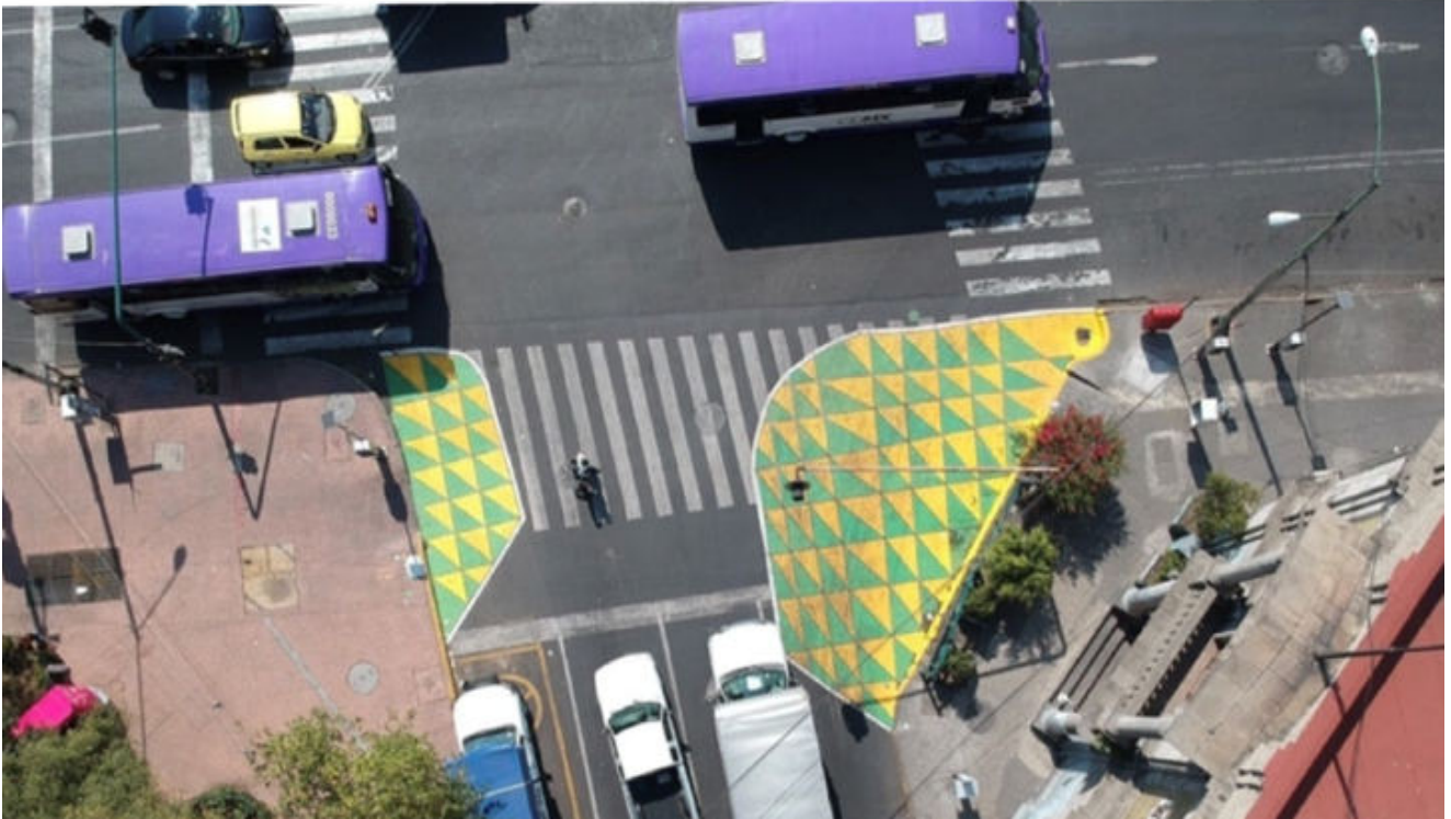
Road crossings made safer through paint markings and 'build outs' in Mexico City. Credit: Institute for Transportation and Development Policy
