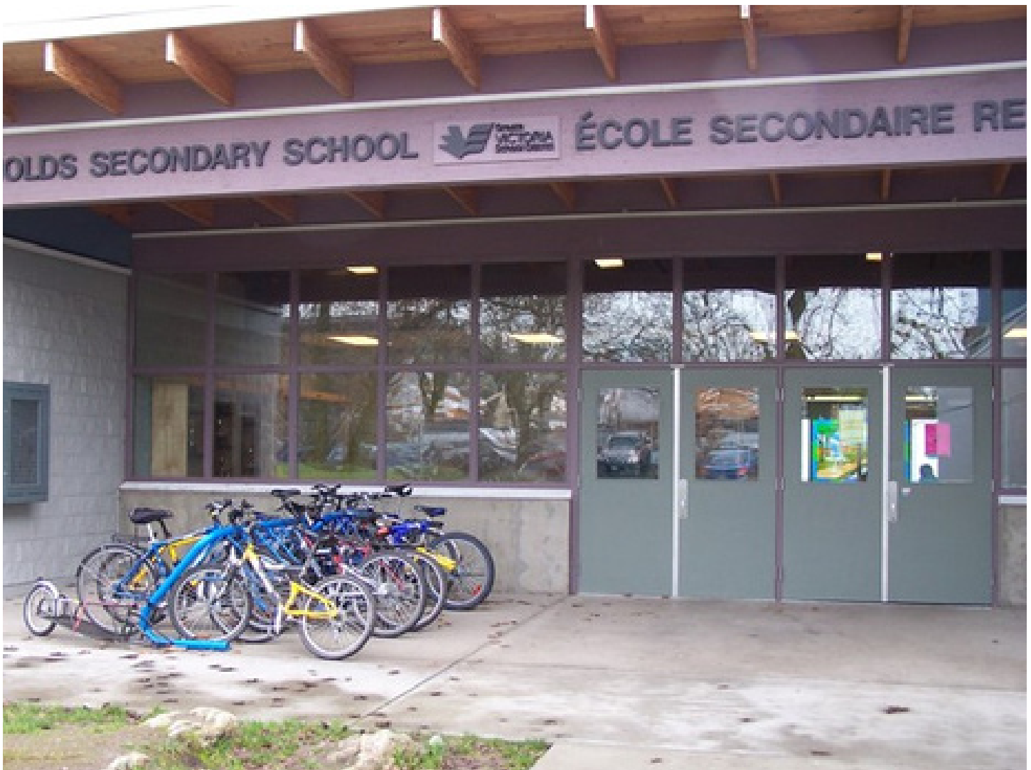
Good quality bicycle parking at a high school in Victoria, B.C. This parking is protected from the weather and in a high traffic area to discourage vandalism and theft. Photo Credit: John Luton.
