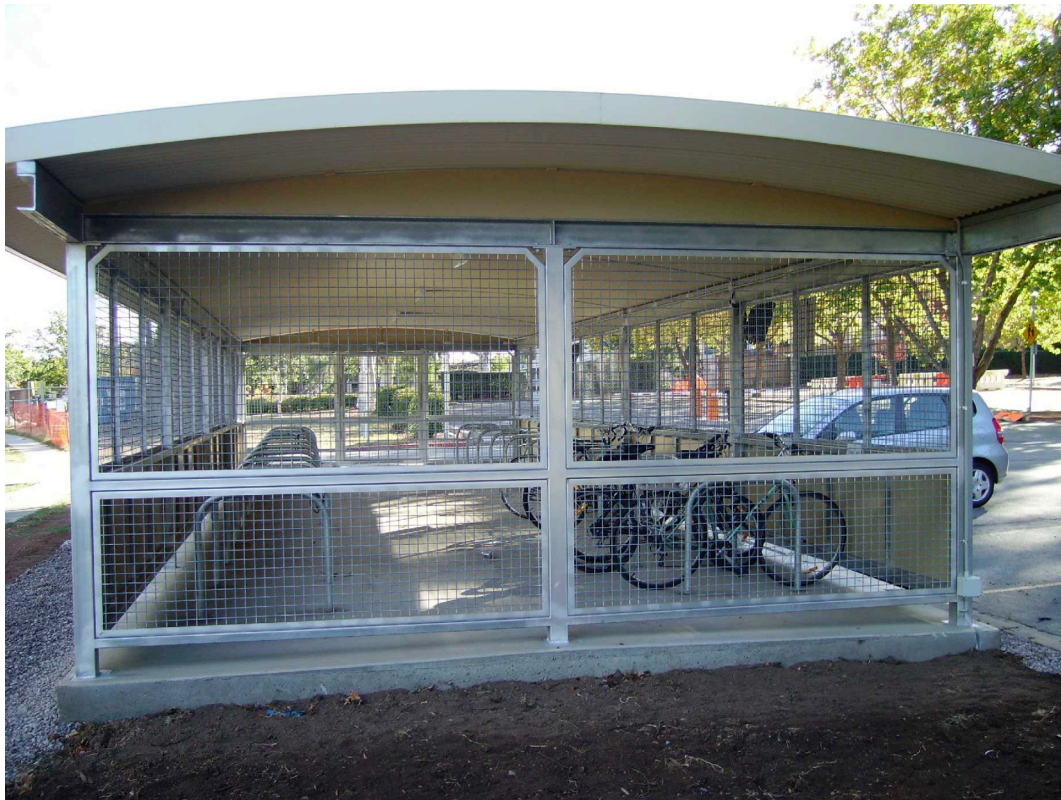
Figure 1 – Example of an Acceptable Bicycle Enclosure
