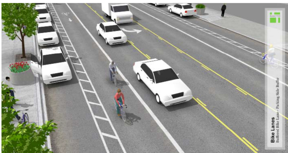
Figura 5 – Buffered bike lane, caso 2
