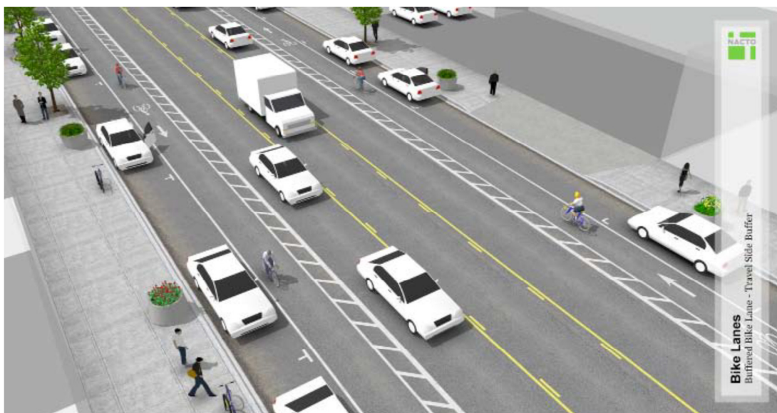
Figura 4 – Buffered bike lane, caso 1
